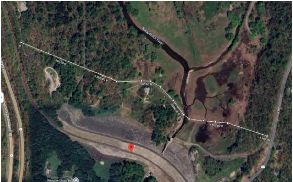
Informational Photo 5: Approximate layout of existing debris boom with measurements (in feet)
