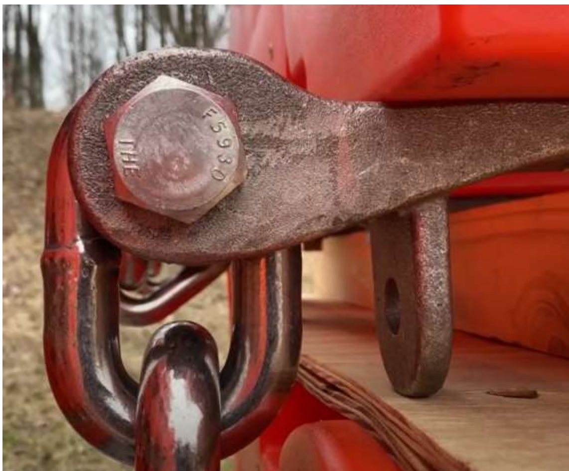
Informational photo 9: Example of new connection hardware (3-part weldless links installed by manufacturer).
