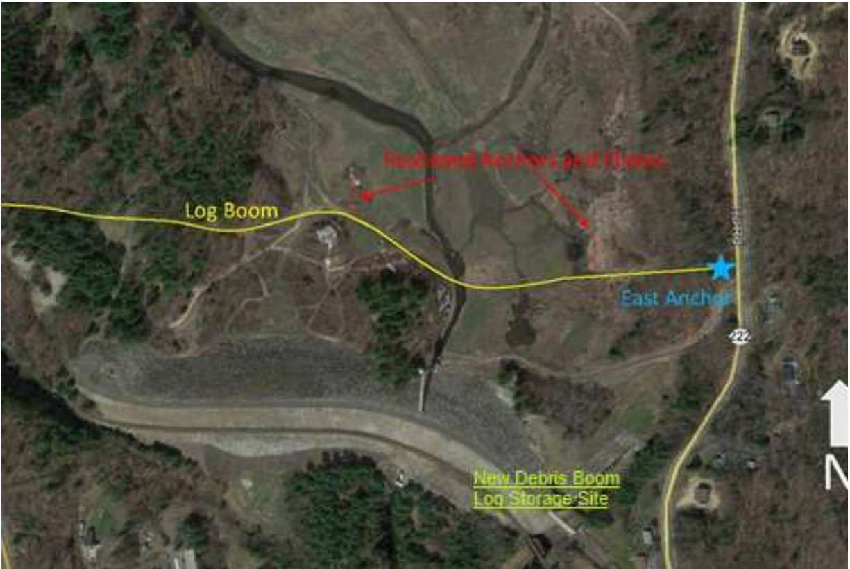
Informational Photo 4 – Layout of entire debris boom, anchors, and center anchor chains.
