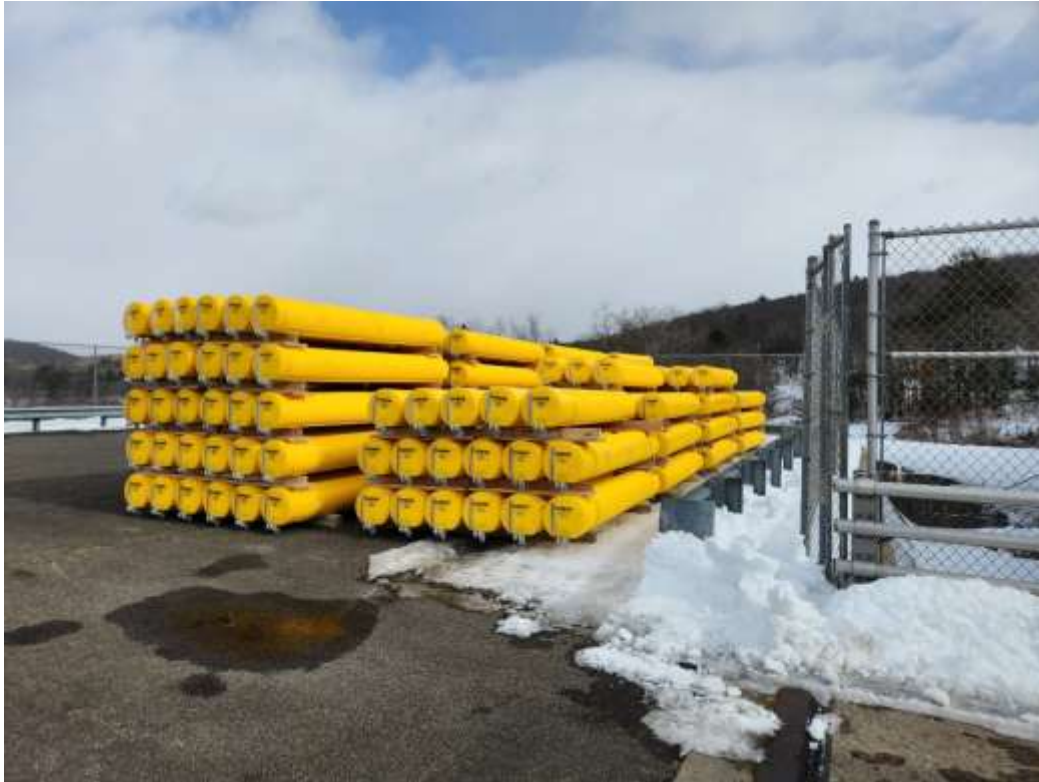
Informational Photo 7: Actual Debris Boom Logs stored at Thomaston Dam
